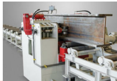
Nắn dầm | Straightening beams
